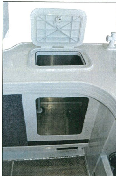
Live bait tanks feature Perspex windows so you can keep an eye on how your livies are travelling.
